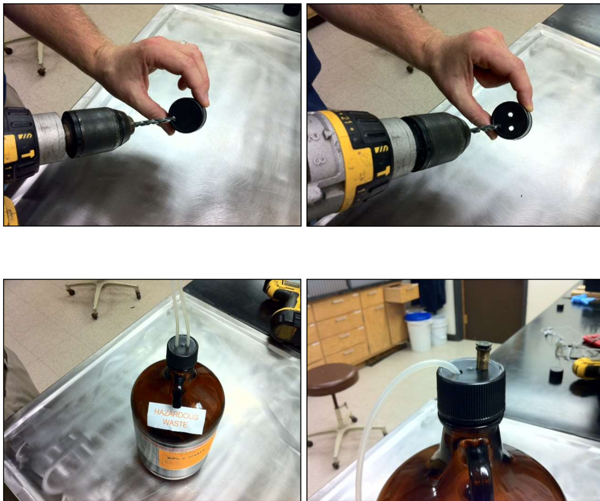
Figure 3 – Examples of Modified Caps for Proper HPLC Waste Collection
