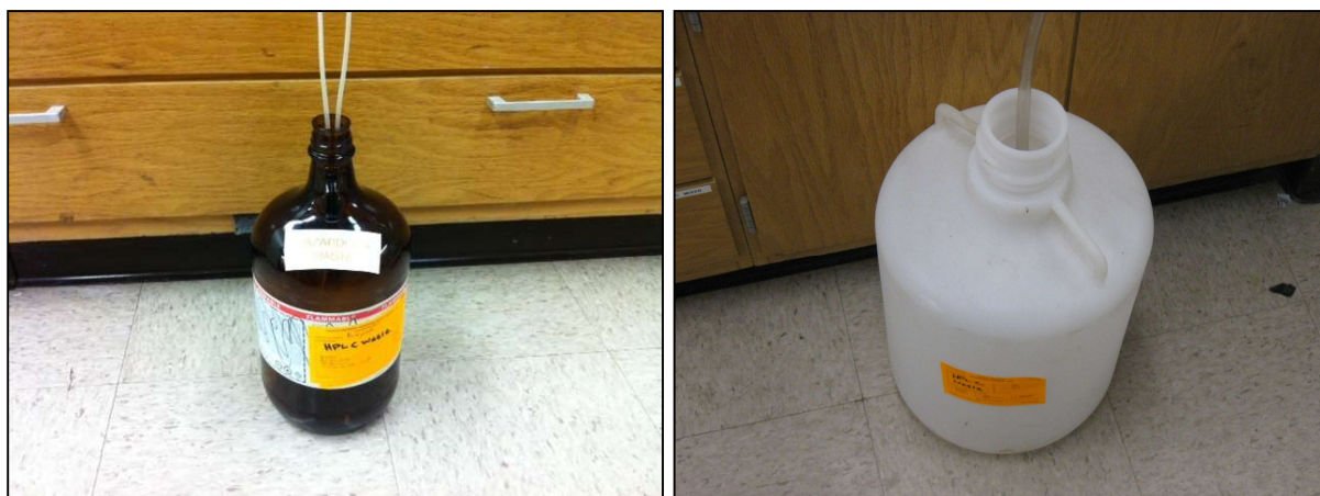
Figure 2 – Improper HPLC Waste Collection Systems (Foil or Parafilm)
