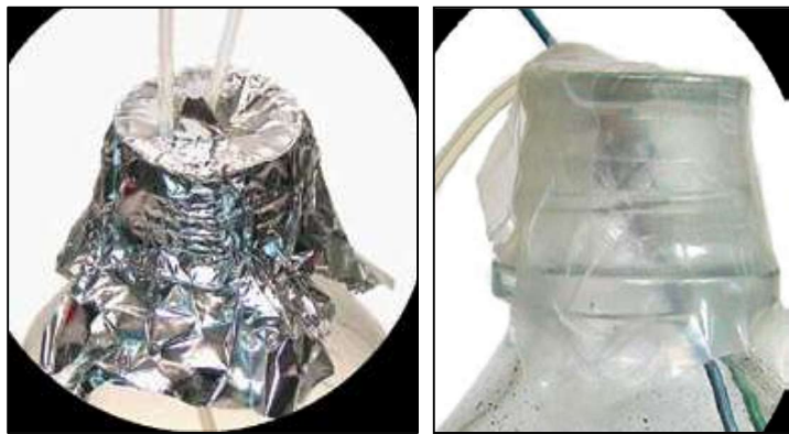
Figure 2 – Improper HPLC Waste Collection Systems (Foil or Parafilm)
