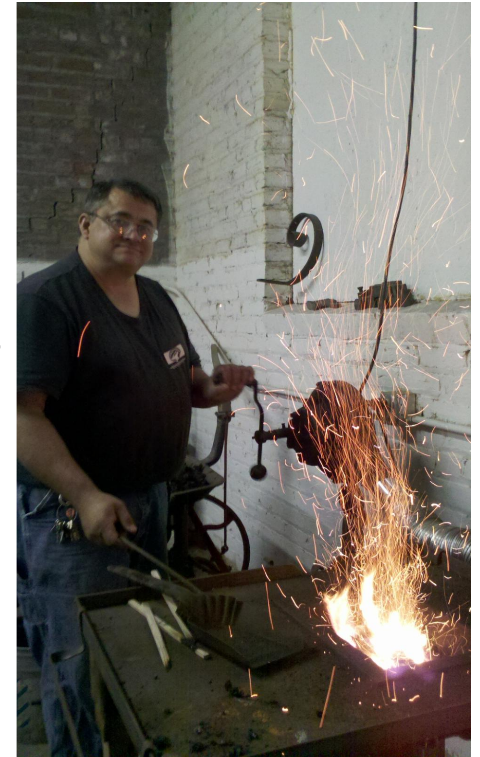
Master Blacksmith Elmo Diaz setting up the coal forge for 3,000 °F work
