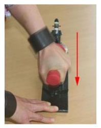
**8.** Now, rotate the lower part of the press counterclockwise until the crimp die (the side with the button back) is located under the press.
