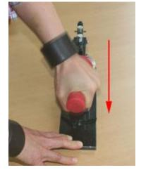
**10.** To create a button with a pin back, take the snap pin and insert it so that its outer edges are underneath the lip of the collet. **Please be careful not to stab yourself.**
