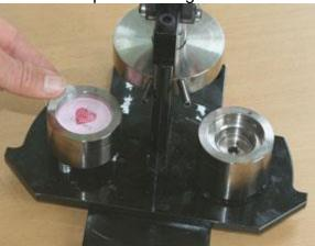
**5.** Place the collet (ring shaped) wide side up into the crimp die (side labeled 2).
