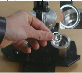
**6.** Rotate the lower part of the press clockwise, so that the pickup die (the part containing the image) is under the press.
