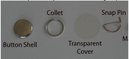
2. To begin assembling the button, place the button shell into the pickup die (labeled 1)
