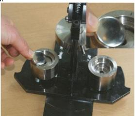
3. Place the image on top of the button shell. Make sure the image faces up.
