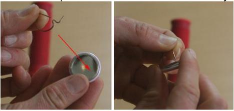
**11.** For large buttons, always make sure image and pin back are aligned in their respective dies.
