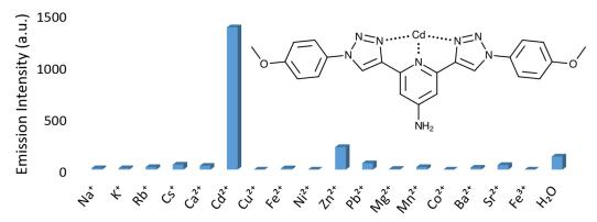
**Figure 4**. Fluorescence emission intensity at 350 nm of a tridentate chelator with NH<sub>2</sub> at the Y<sub>1</sub> position and OCH<sub>3</sub> as X. This analog serves as a cadmium chemosensor.
