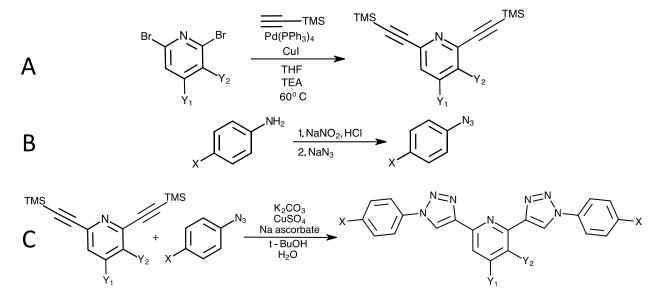
Figure 5. Sonogashira coupling (A), Sandmeyer reaction (B), paired click and deprotection reaction (C)
