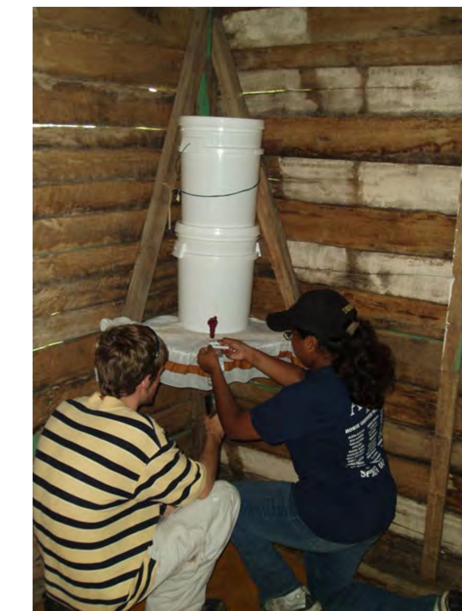
Left: Participants taking a sample from a filter inside a Dominican home. The sample was later taken back to the lab at the ILAC center and processed. The results were then shared with the community so necessary improvements could be made.
