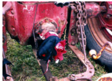
Figure 1. Clothing entangled on bolt on PTO tractor stub shaft
