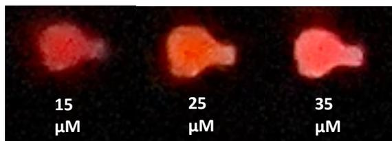
Figure 1. Long exposure images of the oxidation of 5mM  $\text{Ru}(\text{bpy})_3^{2+}$  with increasing concentrations of DBAE
