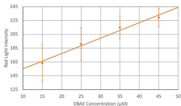
**Figure 4.** Red light intensity Vs. concentration of DBAE in 5 mM  $\text{Ru}(\text{bpy})_3^{2+}$  at a potential of 1.1 V.
