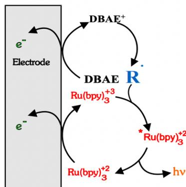
Figure 2. Oxidation-reduction mechanism of  $\text{Ru}(\text{bpy})_3^{2+}$  and DBAE at the surface of an electrode, emitting light.
